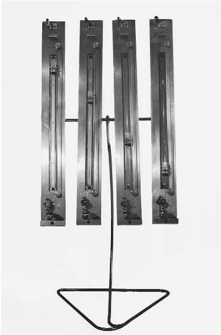
LEMUR's self-playing GuitarBot extends performance capabilities beyond that of a human guitarist.
